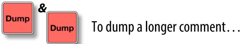
...tap the DUMP button again, while PDM is dumping. Each time you do, PDM will add the preset Dump Size's seconds to the current Dump event. (For example, if you've set a Dump Size of 4 seconds, tapping *twice* will dump 8 seconds.)
