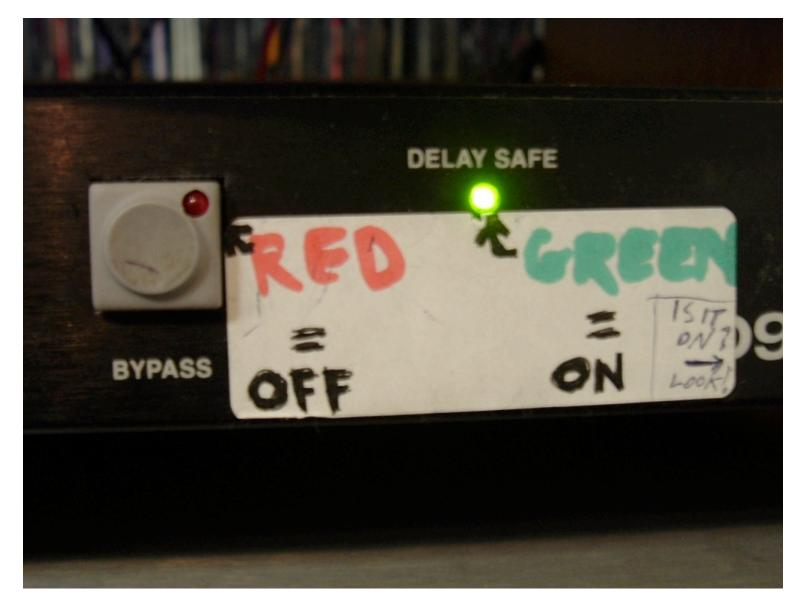
4. If the red light over "Bypass" is on, press the "Bypass" button to activate the delay.
